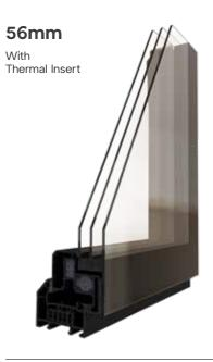
bathroom or kitchen window. Triple glazed thermal reinforced slimline design, ideal for bathroom and kitchen windows exposed to north winds and little sunshine. Five-chamber nylon thermal insert reduces convection, heat loss and steaming up in moist room environments. Perfect for new-build, extension and overexposure replacement. PVC outer, aluminium sash.
