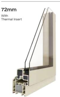
replacement window. Thermal reinforced design, ideal for smaller bathrooms, en-suites or kitchens. Five-chamber nylon thermal insert reduces convection, heat loss and steaming up in moist room environments. 1m maximum span. PVC outer, strong fibreglass inner and frame means steel insert not required.
