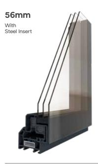
The perfect north-facing, harsh elements large window. Triple glazed steel reinforced slimline design, ideal for larger windows exposed to north winds and little sunshine. Perfect for new-build, extension and overexposure replacement. PVC outer, aluminium sash spanning 1m+.
